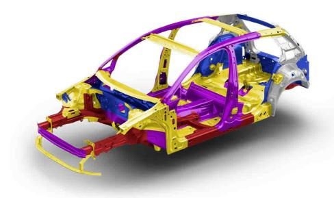
The structure of the all-new Golf R-Line is built with a combination of 5 steel types that increase rigidity and provide optimal safety. At the same time, its structure remains lean and sturdy, so that the overall vehicle is light and carries itself effortlessly. The result? You'll feel a more agile, precise, and efficient driving experience.
